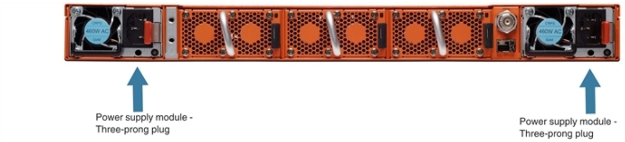
Figure 2 Connecting AC Power (GigaVUE-HCI)
