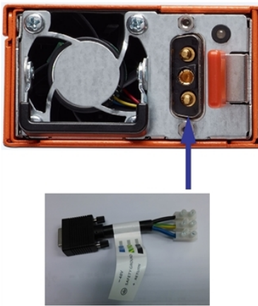
Figure 4 Connecting DC Power Supply Module
